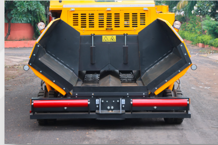
Optimized hopper design for smoother coordination with truck movement
