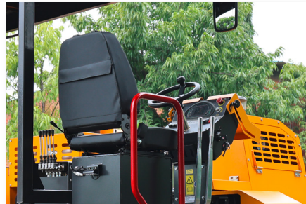
Centrally positioned seat on the drive console for enhanced visibility and improved controls
