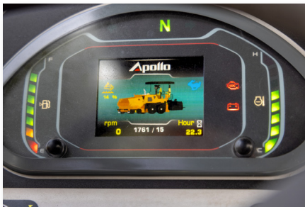
New and enhanced control cluster featuring a colour LCD display
