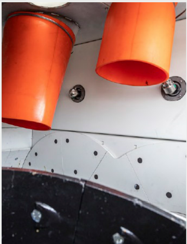
Mixer inlet for cement with the optional silica inlet and mixer cleaning system
