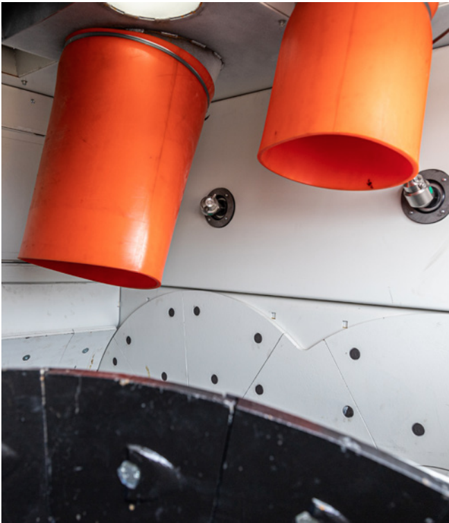
Mixer inlet for cement with the options silica inlet and mixer cleaning system
