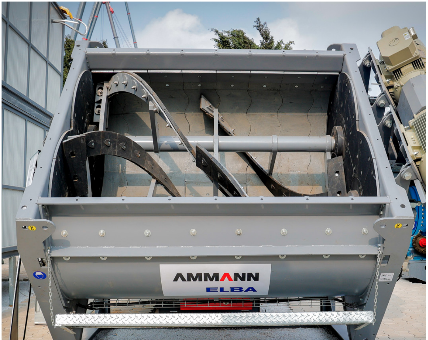
Twin shaft spiral mixer 3 m³.
