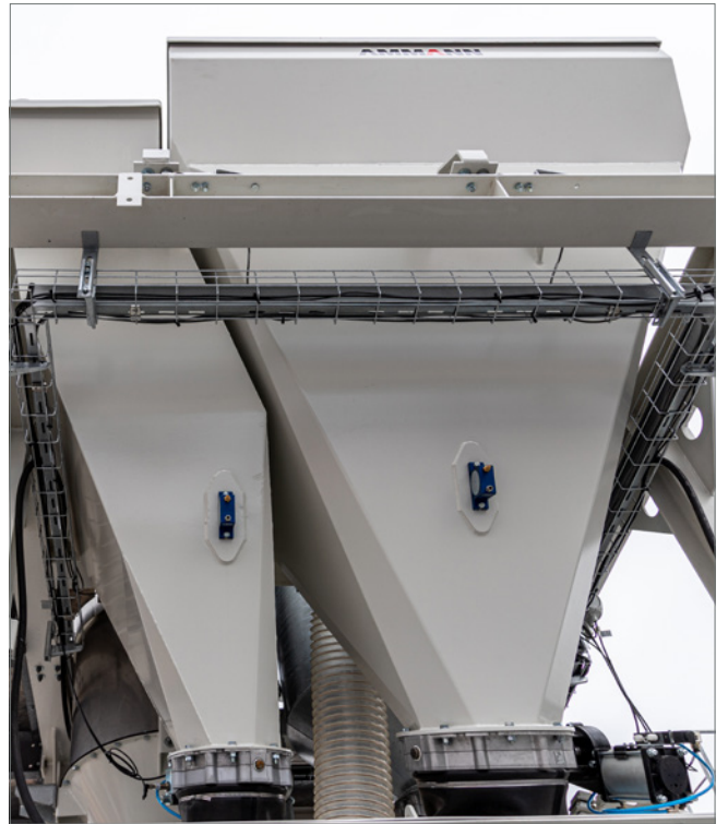
Weighing platform with cement weigher and optional silica weigher
