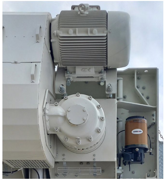
Mixer drive with automatic central greasing system.
