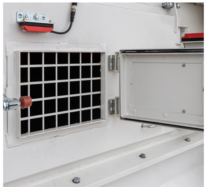
Mixer cleaning flap with integrated inspection hatch contact-protected.
