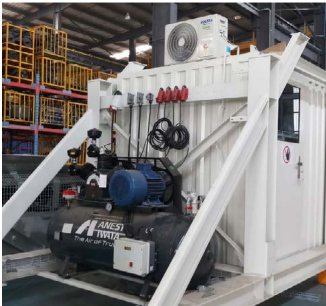
Compact mixing plant: Integrated compressed air system, water connection, pluggable electrical connection points for the linear bin and as option the warm/chilled water connection.
