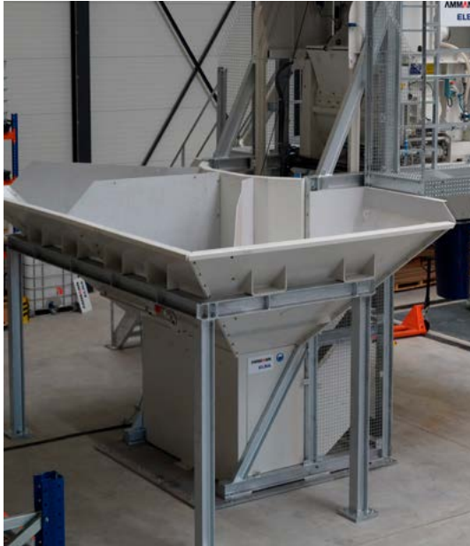
Pocket star with 4 x 2.5 m 3 volume for aggregate storage with integrated batching box.
