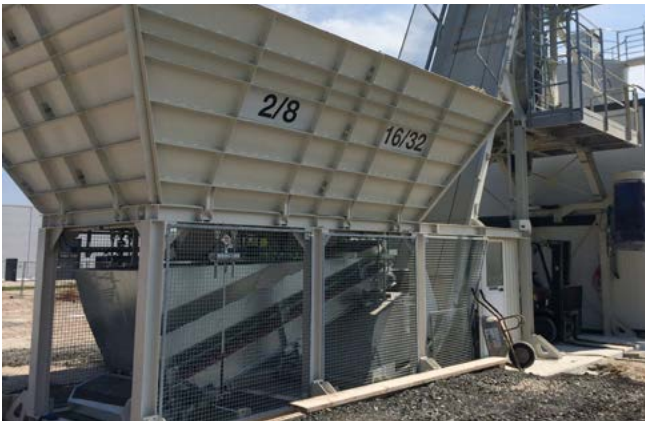
Compact aggregates bin with integrated weighing conveyor belt.
