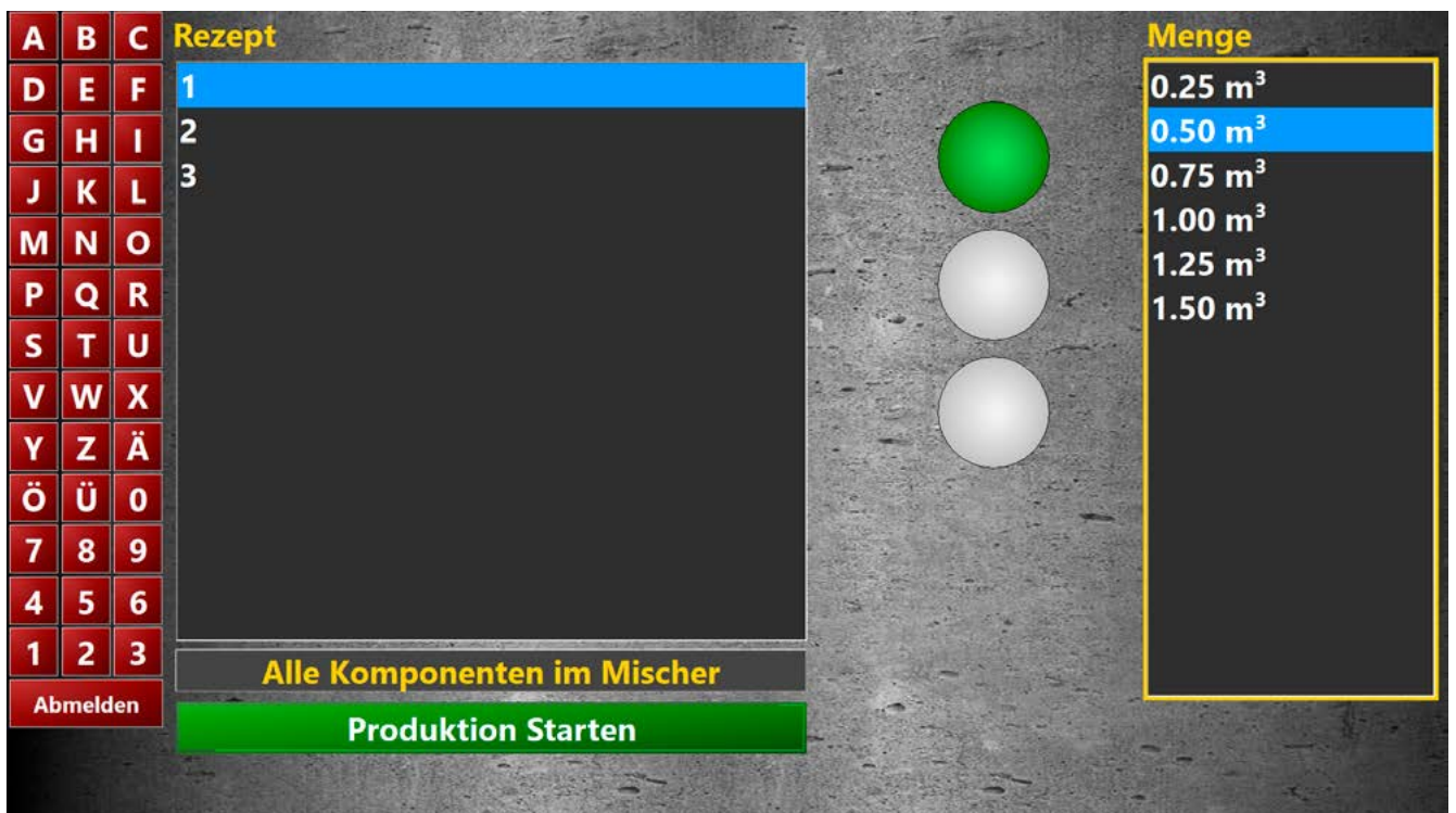
Extremely simple operation via touchscreen with the user dialog and additional traffic light display. As option available, operation via QR code.
