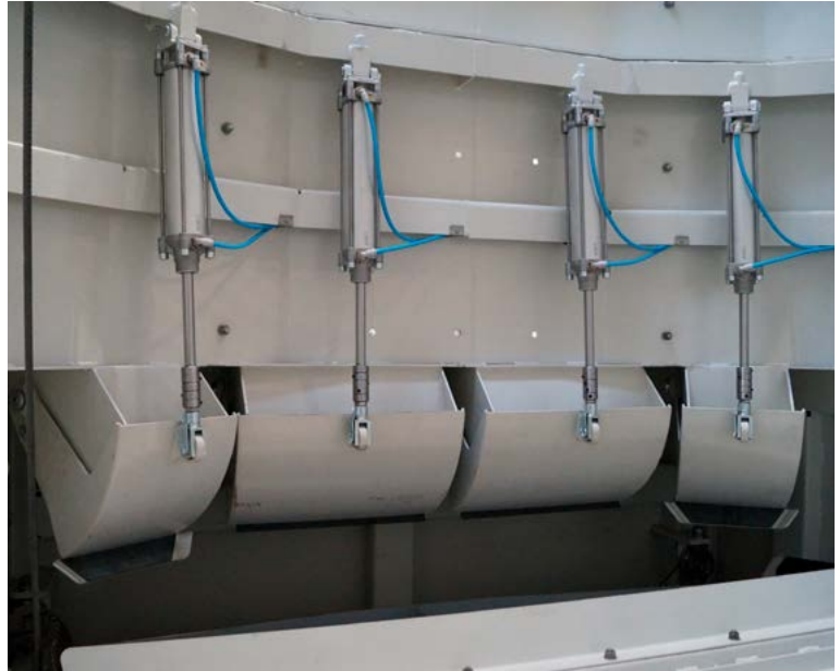
Batching box with built-in pneumatically operated dosing gates and 1500 kg aggregate weigher.
