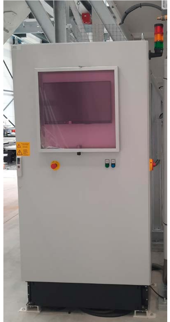
Status display via traffic light system, touch screen operation, optional additive dosing.
