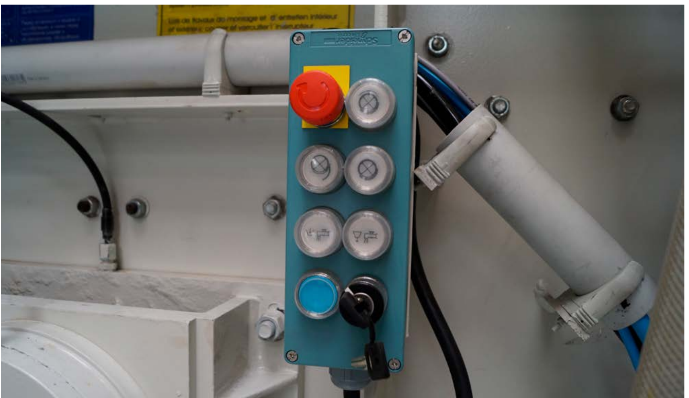
Local mixer operation facilitates maintenance and cleaning work.
