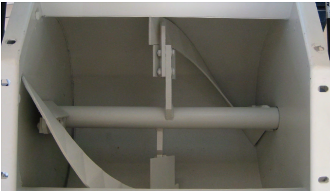
View inside with exchangeable mixing tools.
